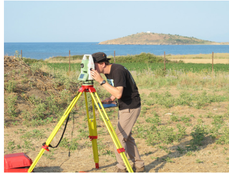
Christian Maines '21 uses the Total Station to plot the location of an artifact
